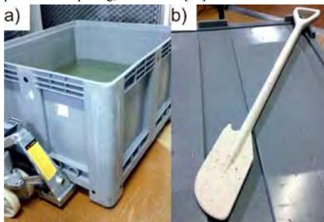
Fig. 1. Tools for manual mixing: a) plastic container, b) paddle mixer.
