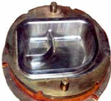
Fig. 2. The mould for a divided tray [21].
