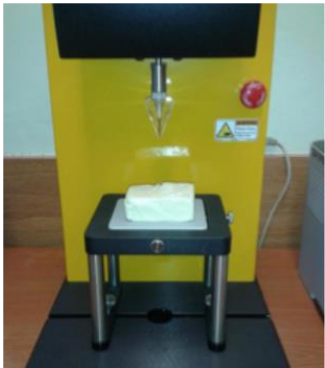
Fig. 2. Testing of the 1st processed cheese sample using a texture analyzer.
