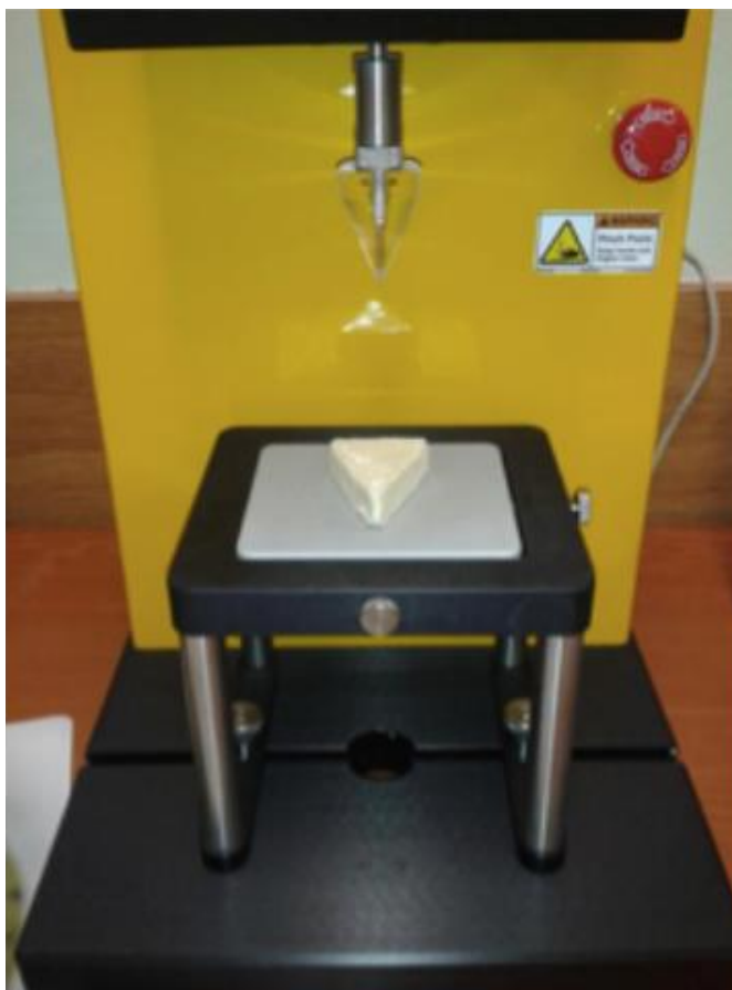
Fig. 5. Testing IV of a processed cheese sample using a texture analyzer.
